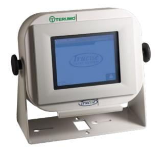
The Trucise system is an electronic documentation and process control device designed to advance the automation of sterile welding while increasing the accuracy and ease of documentation. The Trucise system works with both TSCD and TSCD II sterile tubing welders.
